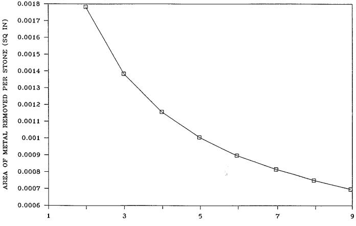
Figure 1. Metal removal vs. grinding speed.
